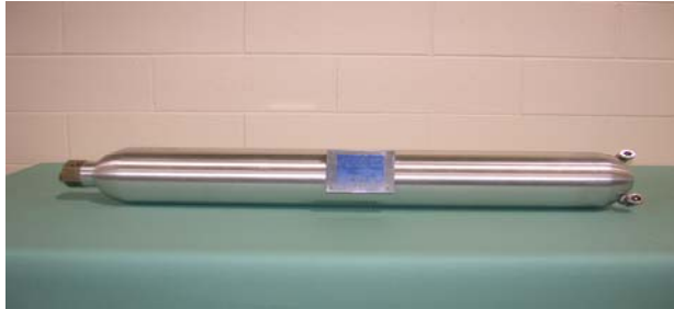
Figure 12. Ovonic aluminum tubular vessel.
